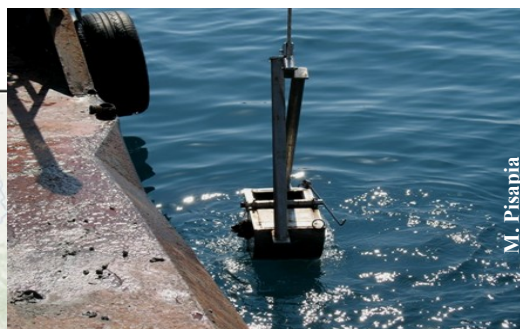
Sediment sampling with Van Veen grab
