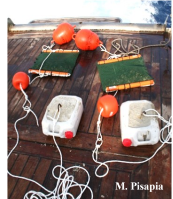
Biomonitoring cages containing mussels
