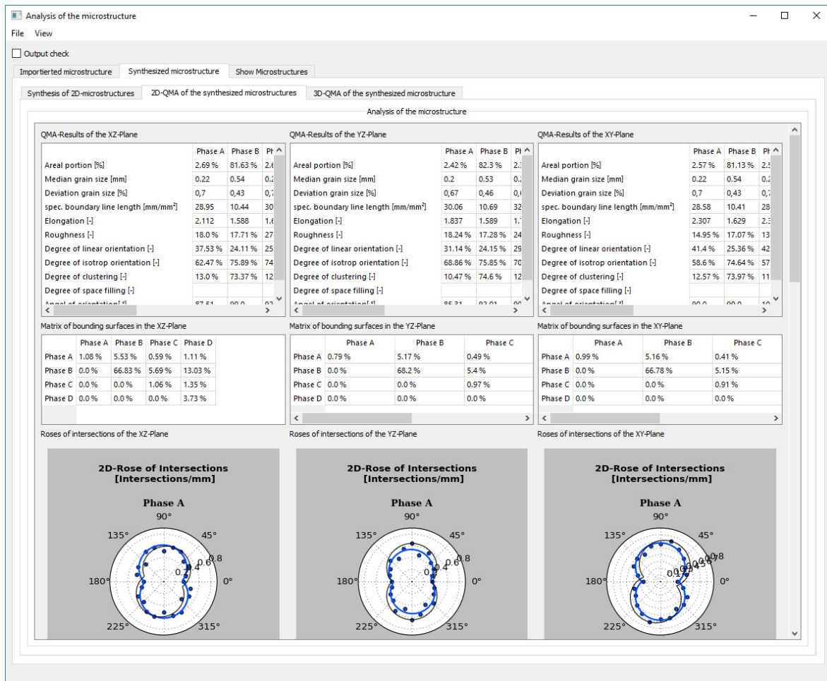
Fig. B.3: Analysis tab with three synthesized two-dimensional microstructures and the associated QMA results
