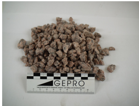
Fig. 4.43: Raw particles of the granite from Meissen in the size fraction 8 to 12.5 mm
