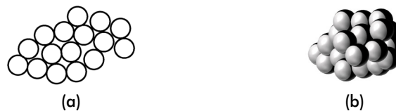
Fig. 2.5: Composite particles: (a) Clump made of bonded circular disks for two-dimensional models; (b) Clump made of bonded spheres for three-dimensional models
