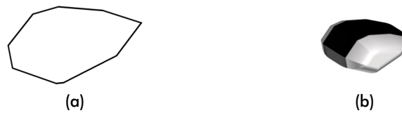
Fig. 2.4: Polygonal particles: (a) Polygon for two-dimensional models; (b) Polyhedron for three-dimensional models
