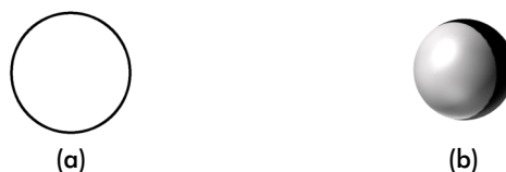
Fig. 2.2: Spherical Particles: (a) Circular disk for two-dimensional models; (b) Sphere for three-dimensional models
