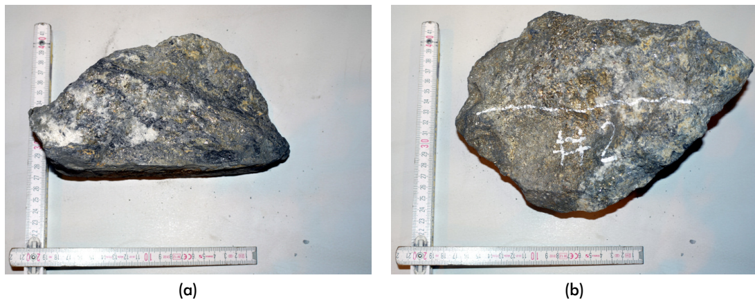
Fig. 4.23: Two sample lumps of the kb-Ore: (a) Sample lump with a mixed microstructure containing both gangue and ore minerals - the intended cutting plane is orthogonal to the view in the lump; (b) Sample lump with a high content of ore minerals - the intended cutting plane, which is marked by the white line, is parallel to the view
