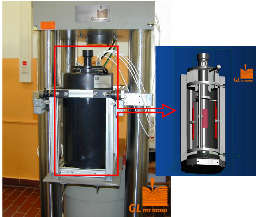
Figure 3.1 DBT A50-80-180 triaxial cell for hydro-thermo-mechanical coupled testing
