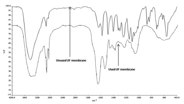
Fig. 3 - FTIR spectra of unused (pristine) and used UF membrane in the present study
