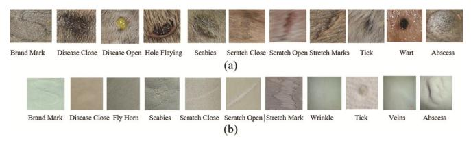
Fig. 1 — Samples of (a) Raw Hides and (b) Wet Blue Leather
