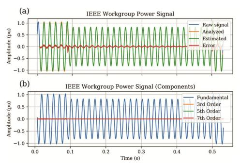
Fig. 2 — (a) Real power signal from IEEE Workgroup, estimated signal by the proposed methodology and estimation error; (b) Real power signal decomposition into fundamental sine-wave and harmonic content of order 3, 5 and 7
