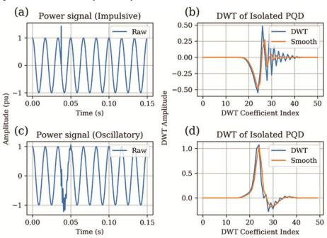
Fig. 1 — (a) Power signal of an impulsive transient; (b) DWT of isolated impulsive transient; (c) Power signal of an oscillatory transient; (d) DWT of isolated oscillatory transient
