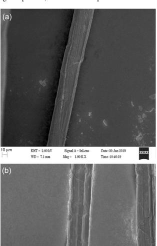
Fig. 2 — SEM Micrographs of (a) raw and (b) HCl treated nettle fibres
