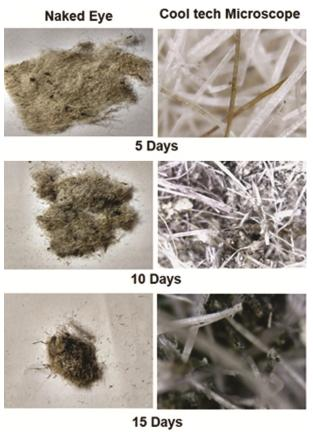
Fig. 4 — Biodegradation of raw nettle fibre after burial in soil
