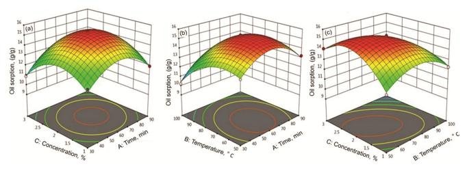
Fig. 1 — (a) Effect of time and concentration, (b) effect of time and temperature, and (c) effect of temperature and concentration on oil absorbency %
