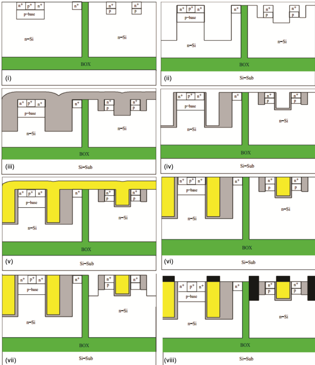
Fig. 2 — Fabrication and design step of the insulator-isolated HVT MOSFET and LVT MOSFET.
