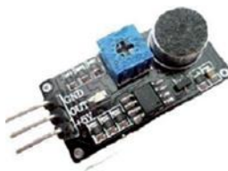
Figure 8. Sound sensor LM393 [60].
