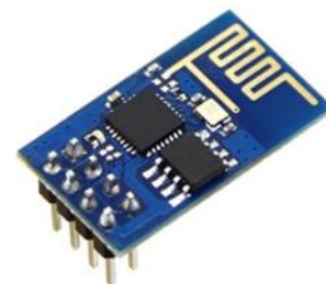
Figure 6. Wi-Fi module ESP8266 [59]
