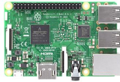
Figure 5. Plate Raspberry Pi [58].
