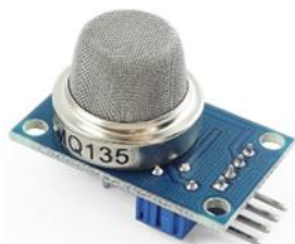
Figure 9. Air quality sensor MQ-135 [61].
