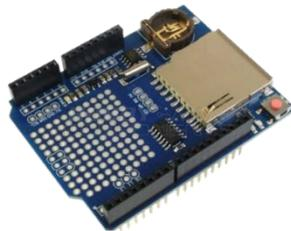
Figura 4 Módulo data logging shield.
