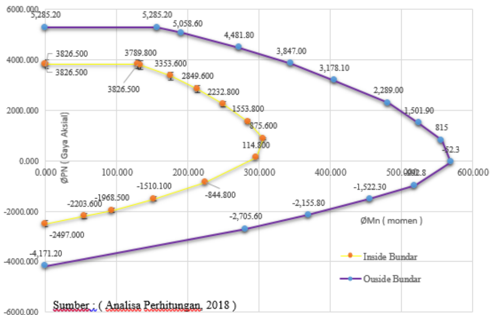
Gambar 8. Superimpose Diagram interaksi kolom komposit inside steel (bundar) dan outside steel (bundar) CSiCOL
