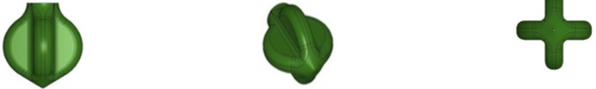
Figure 9: the cut facets pin. The pin has the 90% of the surface extension than each microwell forming the ELISA 96-well microplate.
