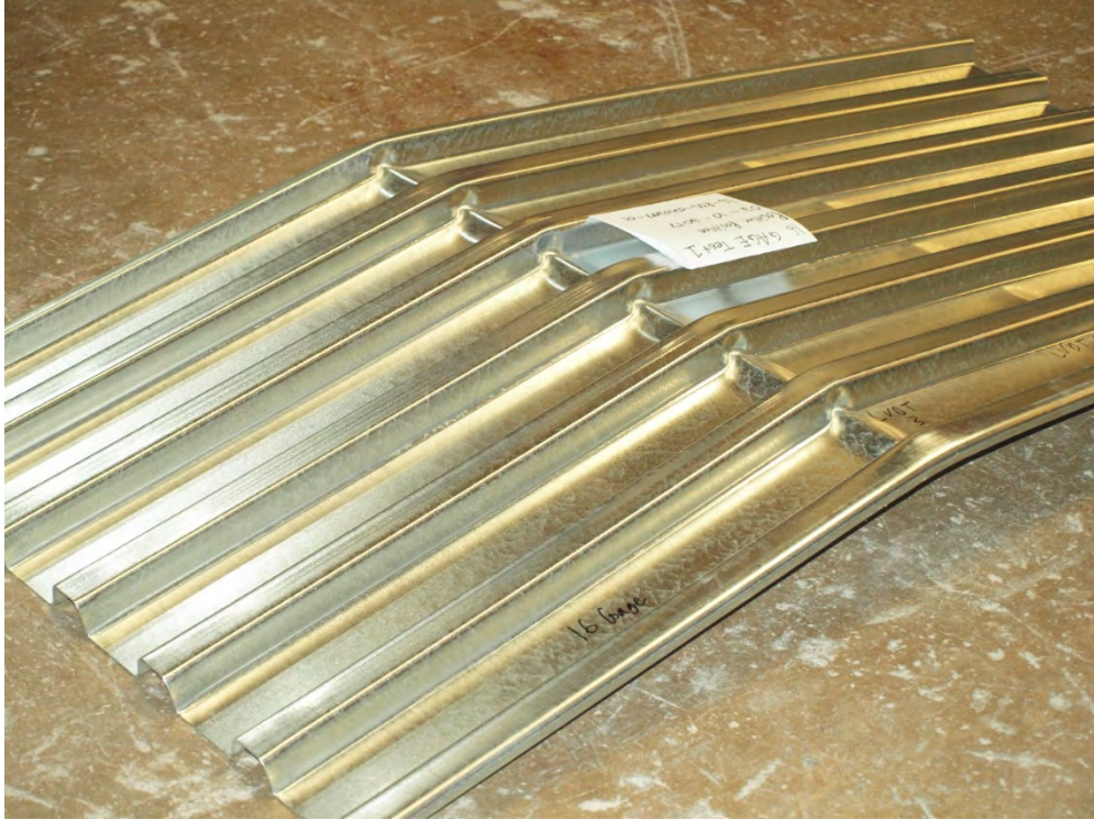
Figure 34: 16 Gage Deck Positive Bending - Final State.
