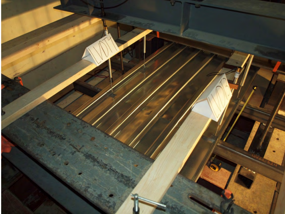
Figure 74: 22 Gage Deck Positive Bending - Initial Buckling.
