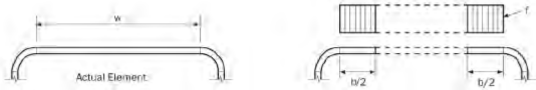
Figure 7: Effective Compression Flange [1].
