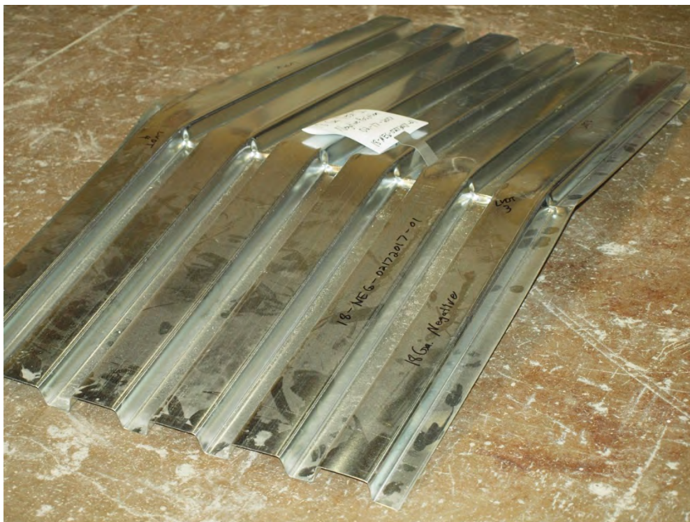
Figure 41: 18 Gage Deck Negative Bending - Final State.
