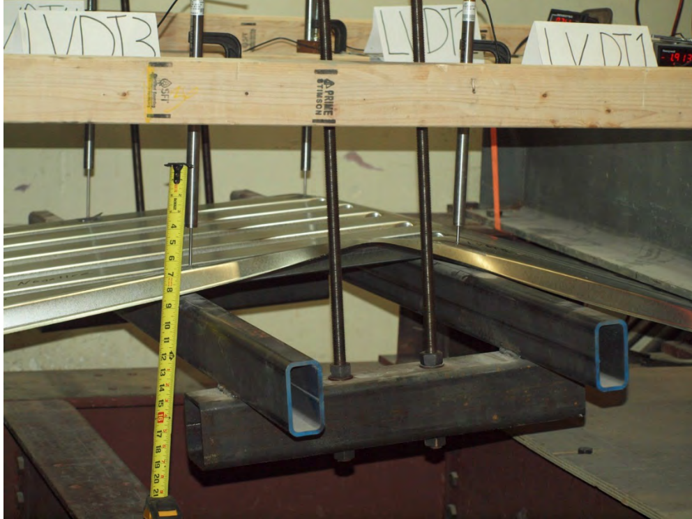
Figure 68: 22 Gage Deck Negative Bending - Final State.
