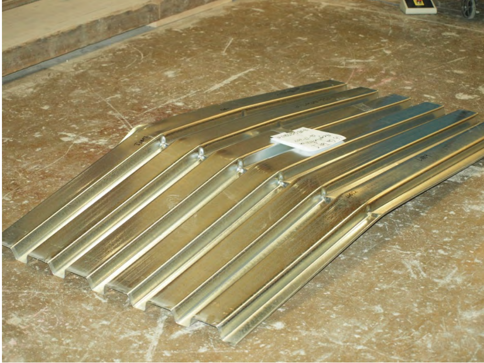
Figure 26: 16 Gage Deck Negative Bending – Specimen Removed.
