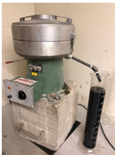
Figure 3. Centrifuge extraction apparatus: extraction of asphalt-solvent solution
