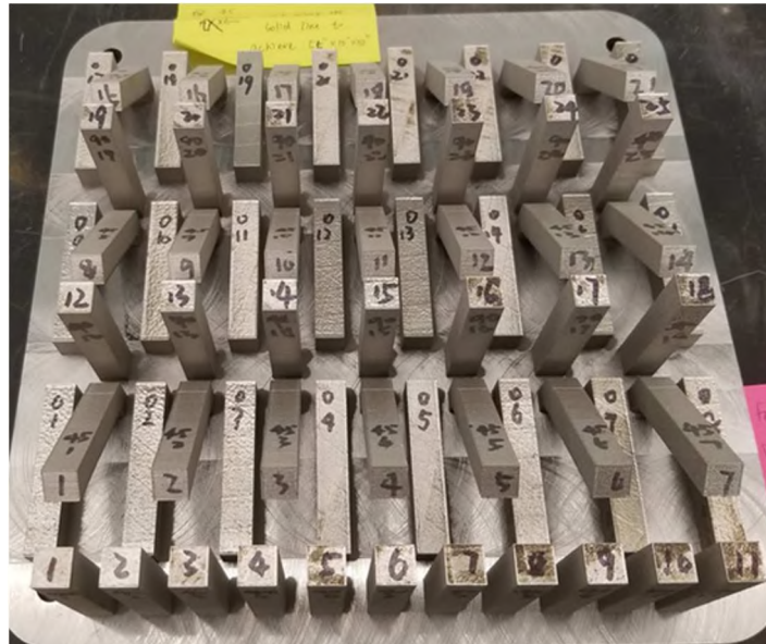
Figure 5. The layout for Build III with toughness optimized parameter in three build orientations.
