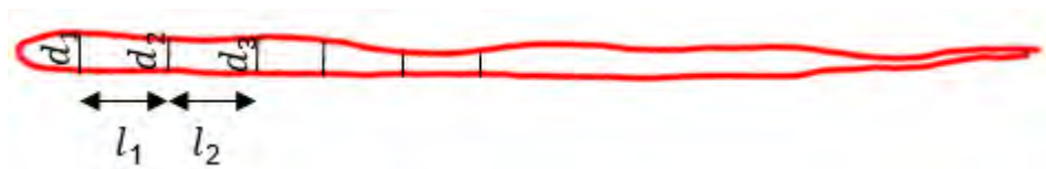
Figure 11. One polyline with calculated d_1 , d_2 , and d_3 values which represent thickness of three segments.
