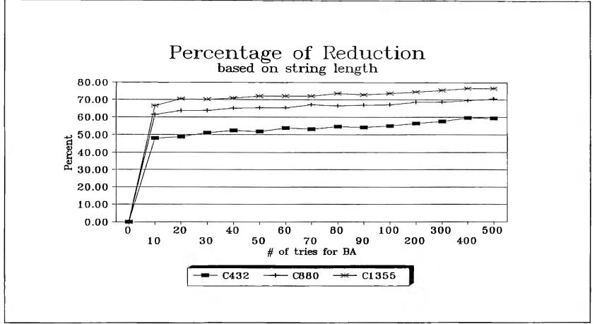
Figure 24. Percentage of reduction in string length for graphs C432, C880, and C1355
