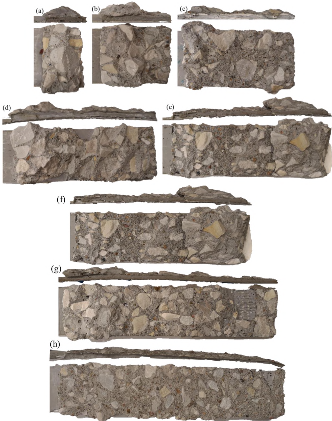
Figure 5. Typical failure mode of single-lap shear test specimens with MD fibers and bonded length of: (a) 30 mm, (b) 60 mm, (c) 90 mm, (d) 120 mm, (e) 150 mm, (f) 180 mm, (g) 210 mm, and (h) 240 mm.
