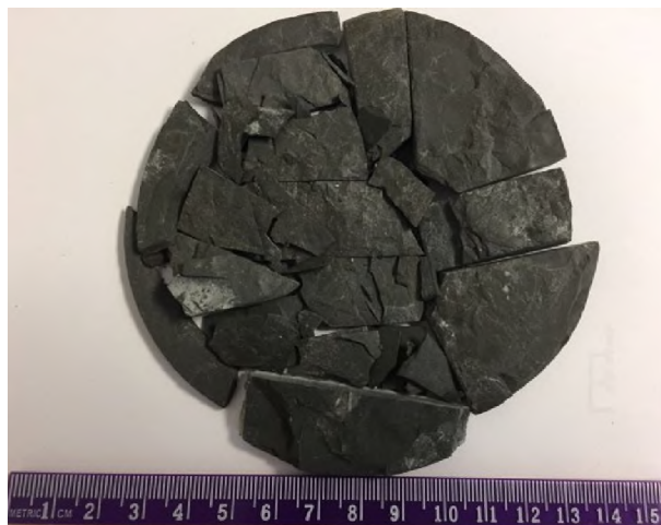
Figure 3. Fragments of the Zubair shale core samples.
