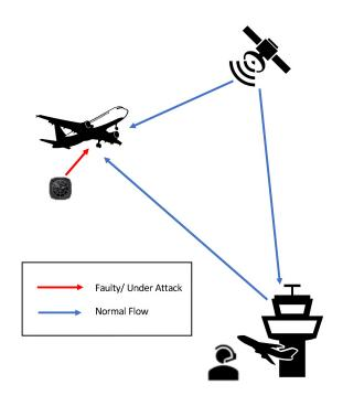
Figure 7.1. ATC Helps to Identify the Faulty Altimeter
