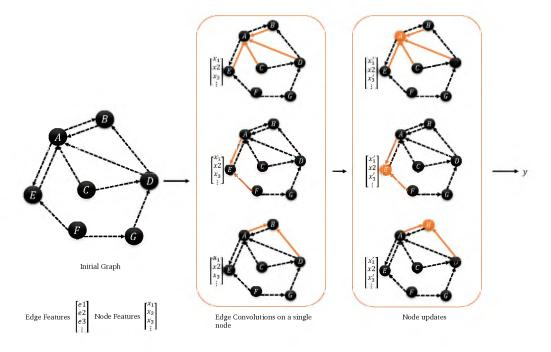
Figure 8.2. MPENN Architecture
