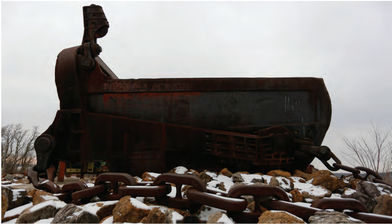
ABOVE | The Big Muskie Bucket sits in Miner's Memorial park, near McConnelsville in Morgan County. The bucket is the last remaining vestige of the Big Muskie, the largest walking dragline ever built.
