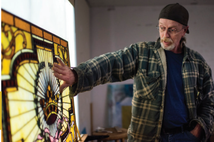
ABOVE | Bernie Evans describes to students the intricate process of soldering grooved lead strips between each piece of cut glass.
