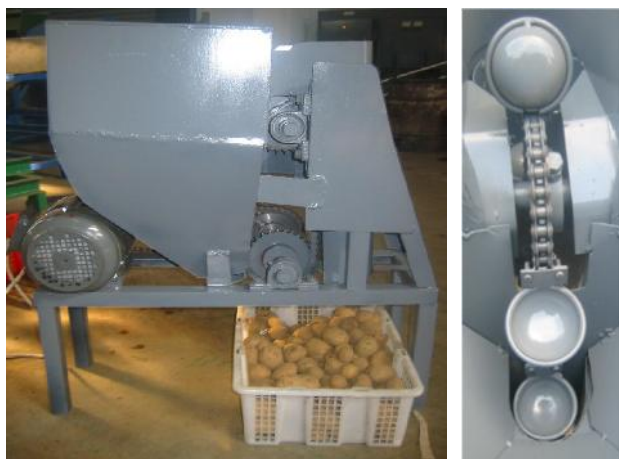
Gambar 2. Apparatus implemen penanam kentang (skala laboratorium)
