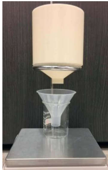
Figure 3.2. Image of the physical hopper used in experiments on discharge dynamics from Arizona State University [11].
