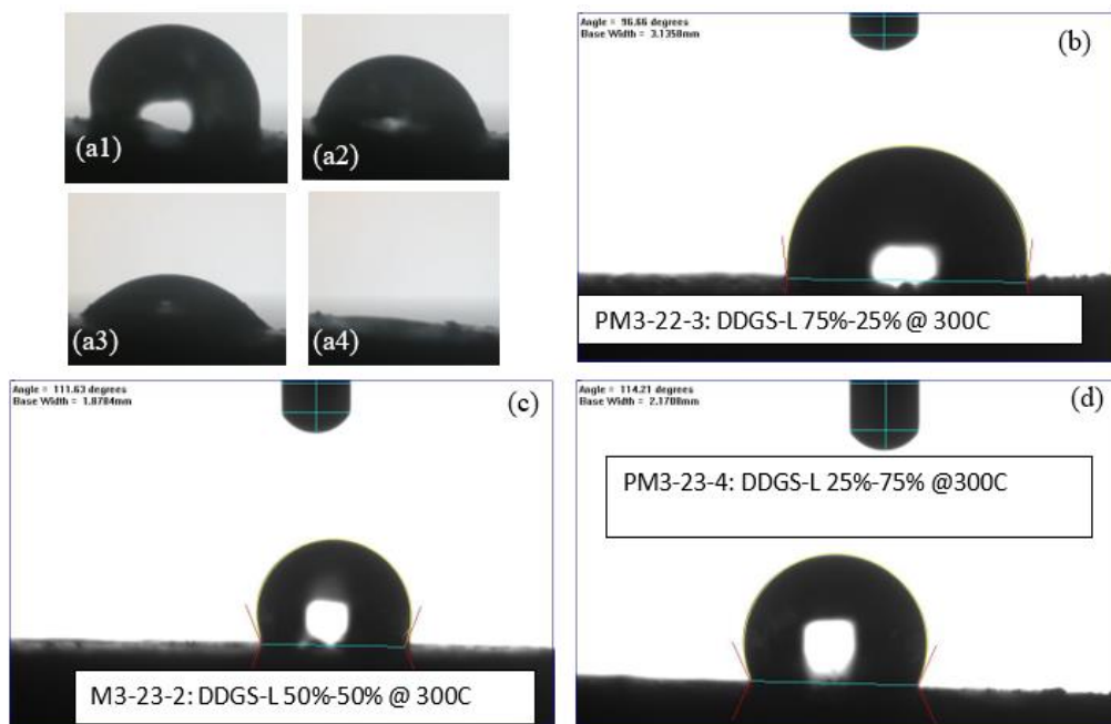
Figure 3.11: Wettability of, (a) DDGS(90)-Lignin(10), (b) DDGS(75)-Lignin(25), (c) DDGS(50)-Lignin(50), and (d) DDGS(25)-Lignin(75) at 300 °C.
