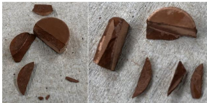
Figure 2.2: Fractured copper samples fabricated at 300 °C.
