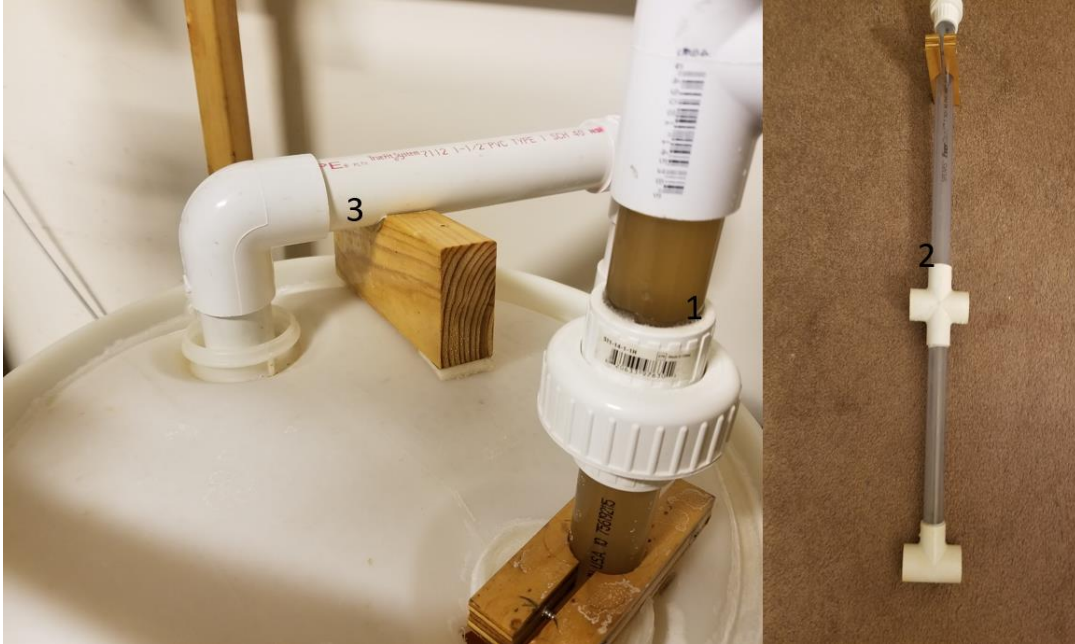
Figure 33. Hydraulic loop return manifold.
