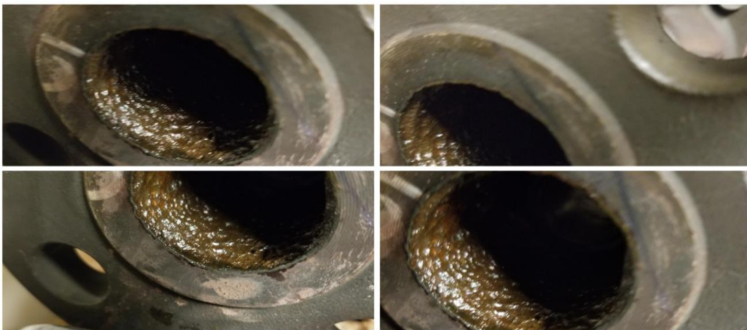
Figure 56. Inlet internal inspection view 240 hours.
