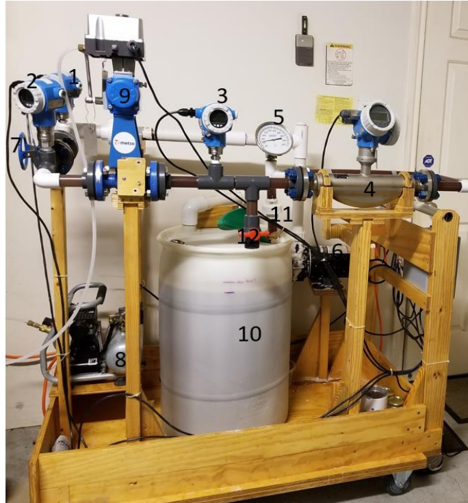
Figure 32. Experimental hydraulic loop system set up.
