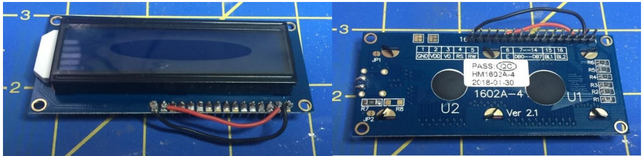
Fig. 3.8. Front and back image of the HD44780 LCD display, with the test pins and voltage input pins successfully soldered/connected and ready for breadboard testing.
