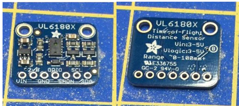
Fig. 3.22. Front (left) and back (right) image of the VL6180X TOF and lux sensor.
