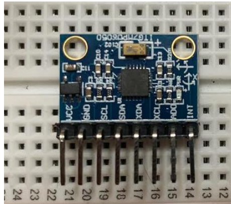
Fig. 5.6. Front image of the GY-521 3-axis accelerometer to be used for precise vibration sensing when paired with a 3D printed PV-embedded airfoil. For more details, the reader is referred to [72].
