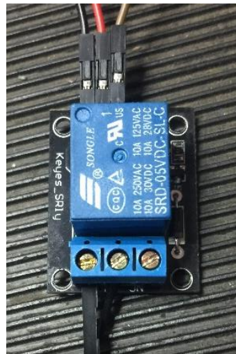
Fig. 3.14. Image of the SRD-05VDC-SL-C assembled serial relay driver used in the ECMS.
