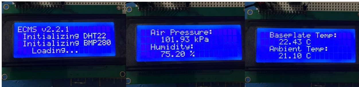
Fig. 3.11. Image showing the startup menu for a sample version of the ECMS, where the code initiates the DHT22 and BMP280 sensors to tell them to start collecting data. The data is broken up into a slideshow presentation where each screen, shown in the middle and right image, stays up for 2 seconds. Setup allows user to monitor air pressure (in kPa), relative humidity (in percent), the baseplate and ambient temperatures (°C).
