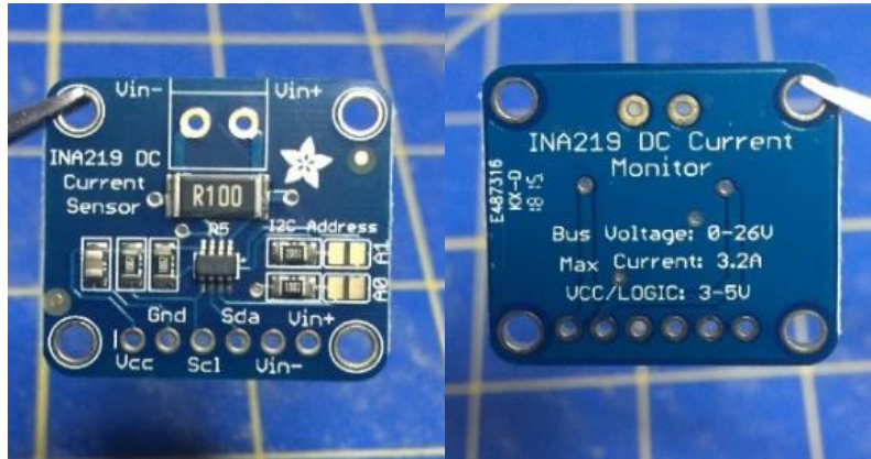
Fig. 3.34. Front (left) and backside image (right) of the INA219 board without headers or pins soldered. The INA219 is directly connected to the positive terminal of the solar panel where the device will measure the current across the 0.1-ohm resistor (R5). For more details, the reader is referred to [63].
