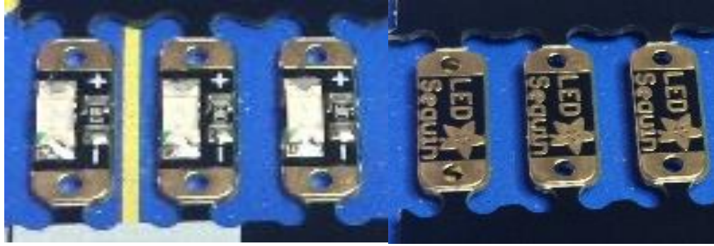
Fig. 3.20. Front (left) and back (right) image of the LED sequins used for the artificial sun to stimulate the solar cells.
