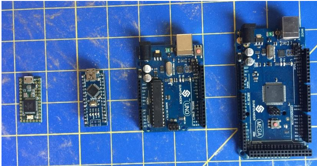
Fig. 3.4. Stacked microcontrollers (from left to right), the Teensy 3.2 board, Arduino Nano, Uno R3, and Sunfounder MEGA 328 microcontroller board. For more details, the reader is referred to [83]-[85].
