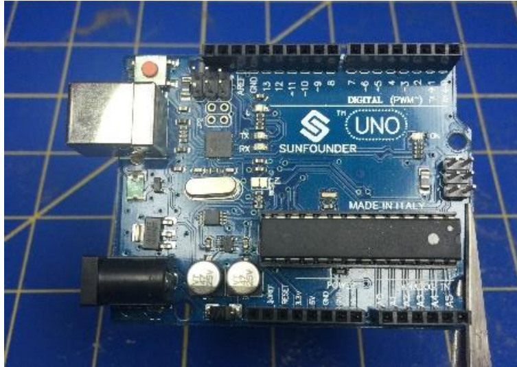
Fig. 3.5. The Italian-made Arduino Uno R3 microcontroller to be used as the central processing unit (CPU) for the BBRs subsystems in prototype testing. Once the code is verified and there are no errors, the more robust ATMEGA328 will replace the R3 as the primary CPU (with the exception of the BAPCS). For more details, the reader is referred to [83].
