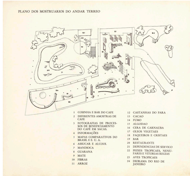
Figure 3.8 Oscar Niemeyer and Lucio Costa. Brazilian Pavilion, site plan from Pavilhão do Brasil: Feira Mundial de Nova York de 1939 . (Source: Biblioteca Nacional Acervo Digital .)
