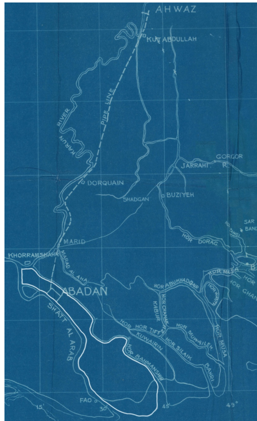
Figure 2.7 The southernmost segment of the oil pipeline. Represented by the dashed line in the map, the pipeline remained very close to the course of the Karun River in the areas where natural terrains permitted.
