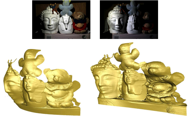
Figure 4. Top: two out of m = 8 RGB images recorded under nearby lightings. Bottom-left: reconstructed shape using the directional lightings and the orthographic projection models. Bottom-right: rendering of the shape reconstructed using the pointwise lightings (18) and the perspective projection (13) models, seen under the same angle.
