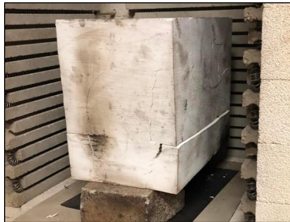
Figure 6. Initial Fluidity Test Block After Burnout
