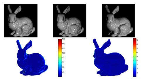
Fig. 11 Test 6: The first row shows the 3 images used to reconstruct the bunny with our method. On the left second row, plot of the color coded normal error for the reconstructed surface using the algorithm in [16] and 10 images. On the right second row, the normal error when using our approach with only the 3 images.
