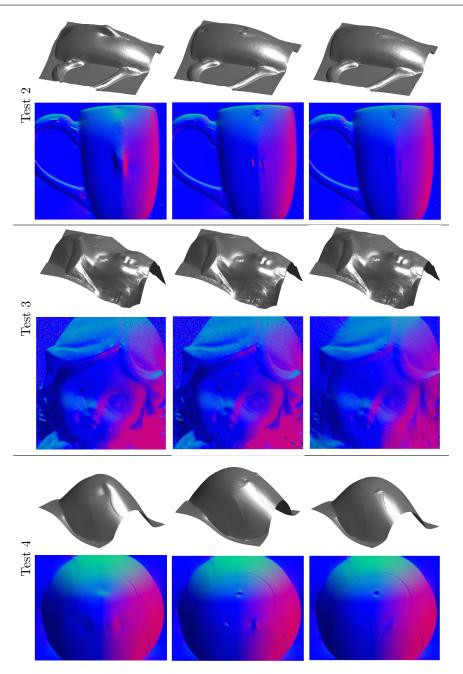
Fig. 8 Reconstructions of Tests 2, 3, 4 corresponding to case A. On the first column, traditional PS approach with global reflection assumed purely diffuse. The second column shows the reconstruction from the diffuse component where the normals of the surface in the highlighted sets have been recovered by inverting the Blinn-Phong shading model. The last column presents the reconstruction obtained by using our method showing visible improvements in the 3D reconstruction and normal map.
