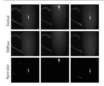
Fig. 5 Test 2: Images of a painted ceramic cup before (first row) and after the reflection separation (second and third row).
