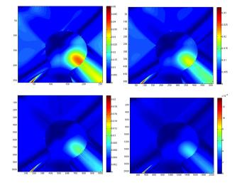
Fig. 14 Test 7: Error map varying the size of the input images starting from  $256 \times 256$  (first row on the letf) to  $2048 \times 2048$  (second row on the right).
