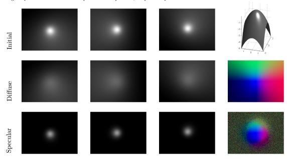
Fig. 4 Test 1: Images of a paraboloid with 1% of Gaussian noise before (first row) and after the reflection separation (second and third row). The last column shows the ground truth on top, the color coded normal map computed by using the diffuse (second row) and the specular (third row) data having respectively 2.032 and 147.72 degrees as maximum angular error with respect to the real normal field.
