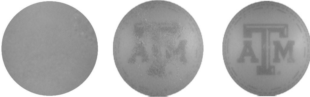
FIG. 1. Increasing transluency of samples with silicate concentration of 12% and SPP concentrations of 0.70%, 0.96%, and 1.5% (left to right)
