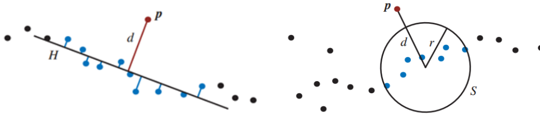
Figure 3: a) The distance ( d ) of an outlier ( p ) from a surface generated by its neighbors ( H ) exceeds a certain threshold. The k - nearest neighbors are highlighted in blue and the H surface is generated based on minimizing the squared distances of k -nearest neighbor points ( \min \sum distance(p, H)^2 ). Distance values ( d ) should be normalized to handle possible noise and surface deviations.
