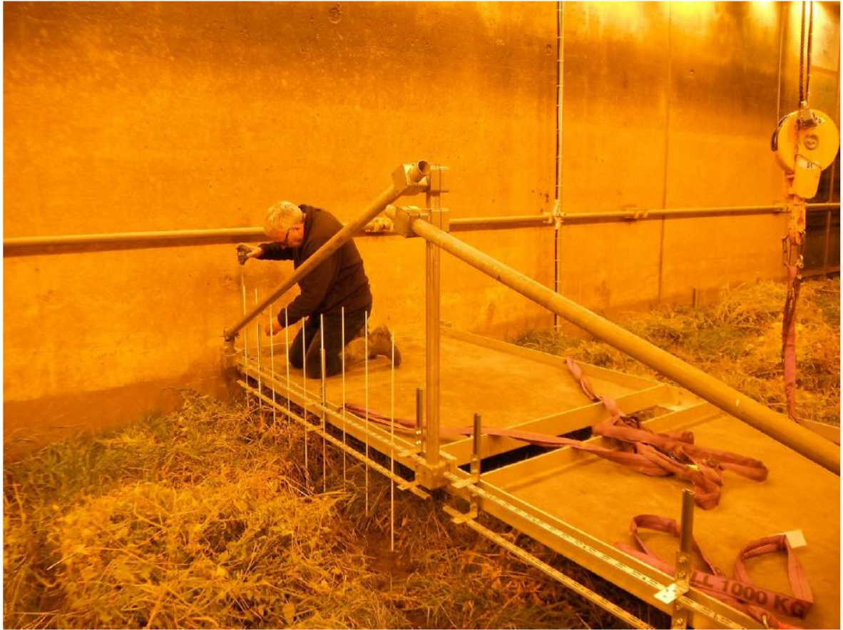
Figure 2: Cross-flume measurement of marsh surface elevation with first 9 pins of pin array deployed from temporary platform keyed into sidewall benchmarks (photo: I Möller)
