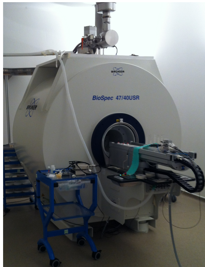
Figure 2.30: Bruker Biospin 4.7T MRI scanner for small animals installed at the WBIC.
