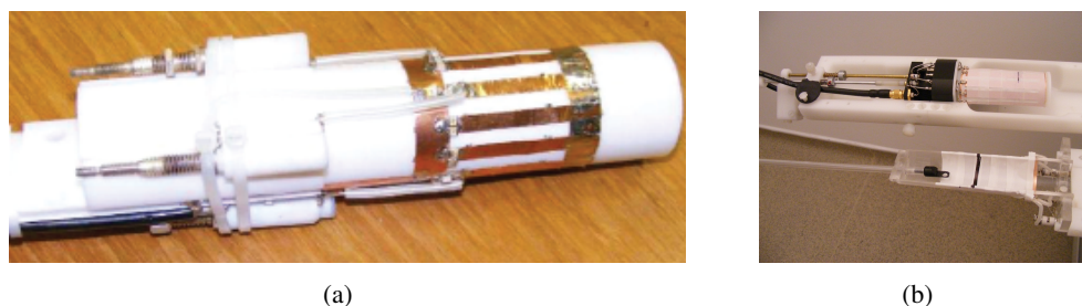
Figure A.3: Custom-made RF coils: (a) transmission coil and (b) mouse head coil. Photos used with permission of Dr Rob Hawkes.
