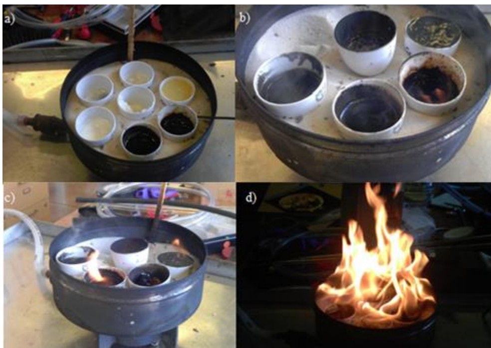
Figure 3.2 Images showing the progression of the pyrolysis stage of the resin-gel synthesis. Image a) shows the crucibles with the waxy solid evenly spaced in the sand bath (the two darker samples had already been heated for some time). Image b) shows the blackening of the samples with heating at 400 °C and spontaneous ignition of one sample. Images c) and d) show the more vigorous stages of the burn.
