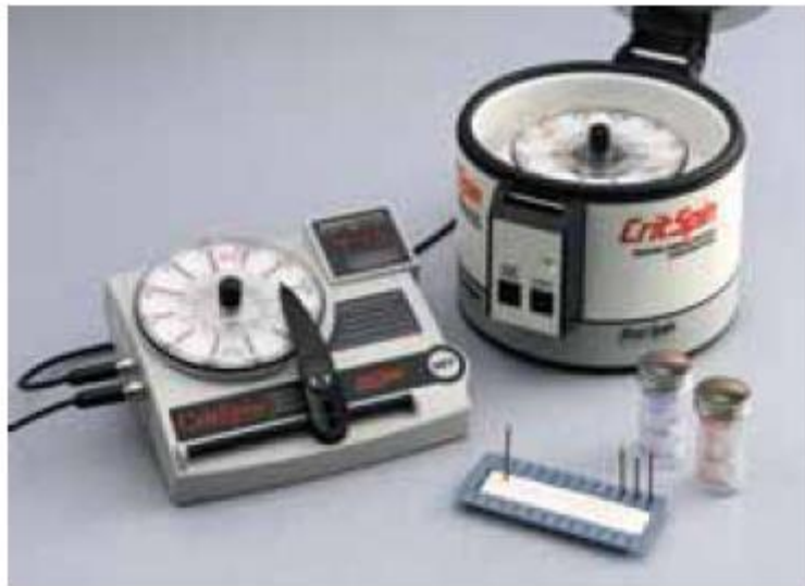
Figure 20.1 Standard microhematocrit centrifuge. Maximum packing time is dependent on a calibrated centrifuge.
