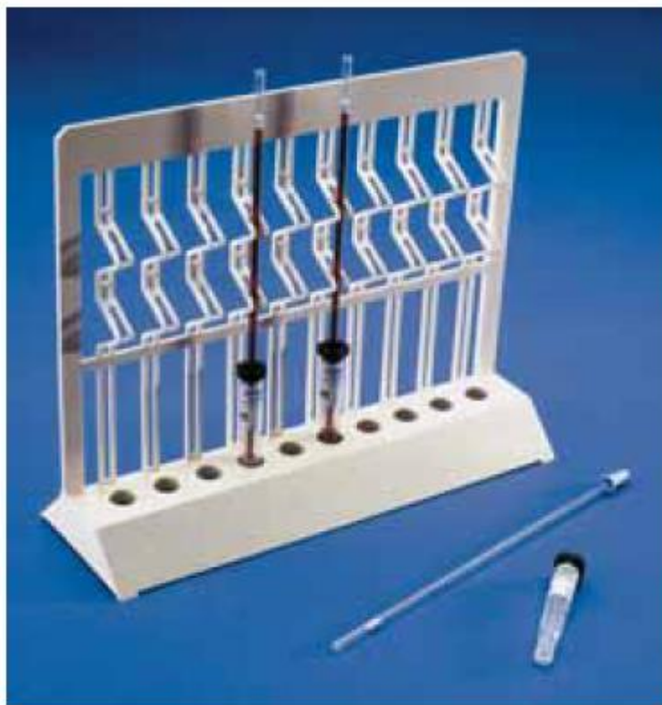
Figure 20.4 Sediplast ESR rack. The sample must be placed on a level surface with no vibration.
