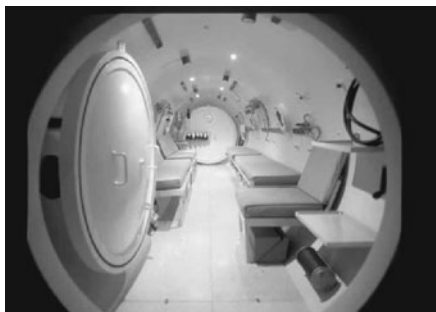
FIG. 130-2 Multiplace chambers. SOURCE: Adapted from http://www.sechristind.com/ .
