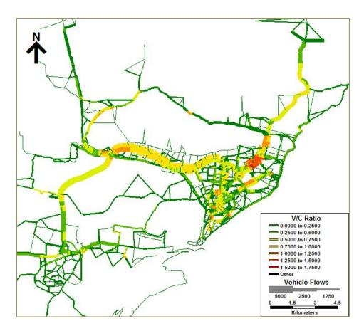
Figure 25 Output of traffic assignment in TransCAD
