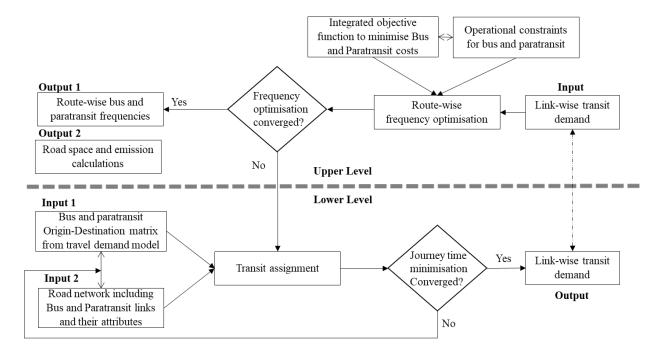
Figure 5 Bi-level model developed for transit assignment and frequency optimisation
