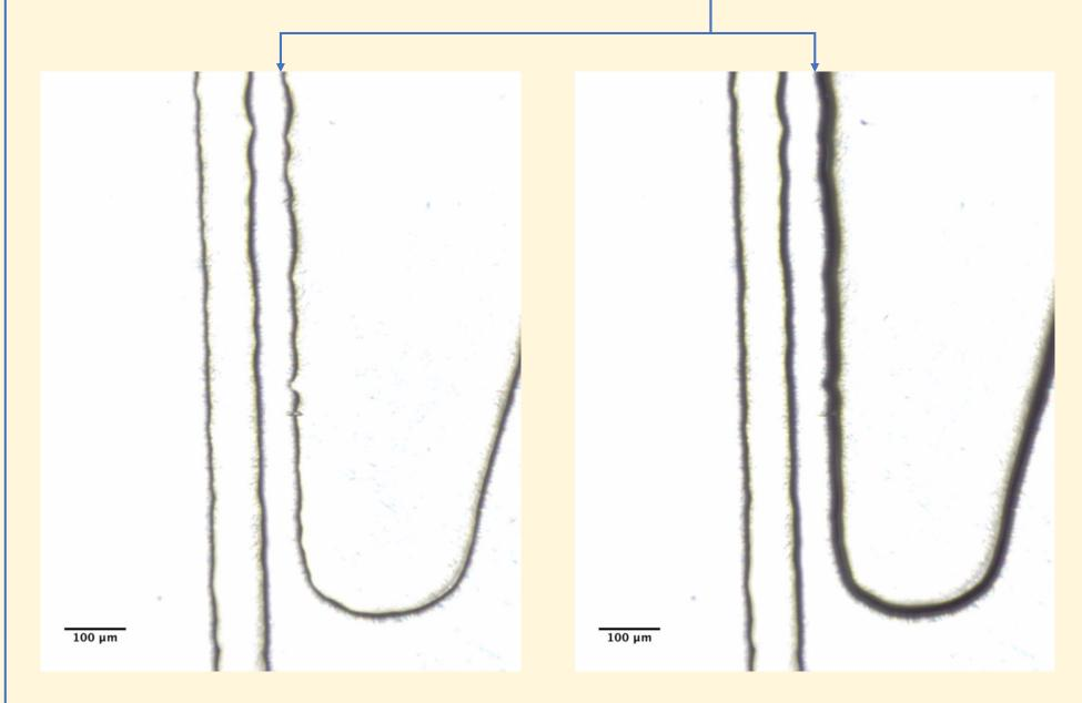
(Left) An unpressurized plunger < 100 μm from a channel. (Right) The same plunger with pressure applied. The bolder outline is from a shift out of focus due to upwards elastic deformation of the plunger.
