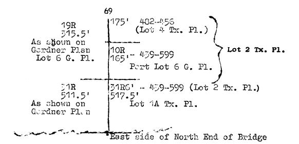
Both the Gardner Plan and the Tax Plan agree that the distance from the bridge to the North Side of the Lewy Farm is 200 rods along the Houlton Road. On the right side of the line are shown the lots and their frontage on the road as they should appear on the Tax Plan. On the left side is shown the Gardner Plan lots and their frontage. The source for each frontage is given.
