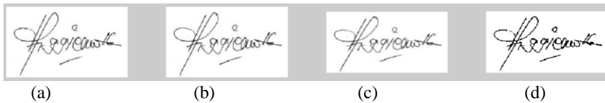
Gambar 4. a) citra asli, b) citra grayscale, c) citra resize, d) citra biner
