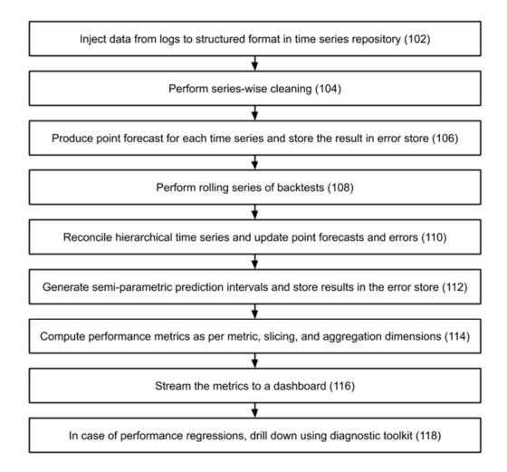
Fig. 2: A forecasting process for capacity planning
