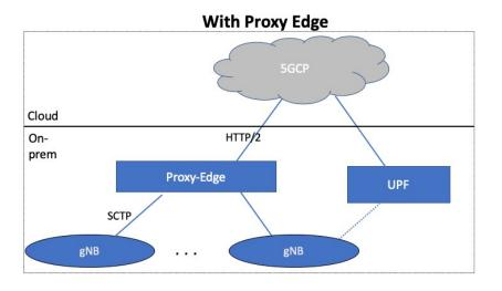
Figure 2 – Architecture with Proxy Edge Function
