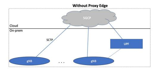
Figure 1 – Architecture without Proxy Edge Function
