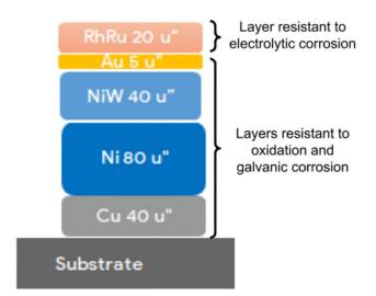
Fig. 2: Corrosion resistant plating configuration for connector pin
