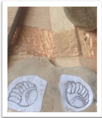
Fig.20 Pasting of designs to cut
