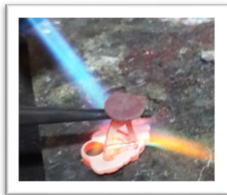
Fig. 30 Soldering of the locking mechanism
