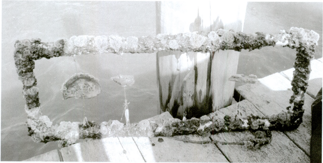
Figure 3: An array retrieved after being submerged for two weeks. Plates were suspended with monofilament to isolate the plates from possible overgrowth by organisms on the rack. They were attached to the rack with rubber bands to maintain tension and plate stability.
