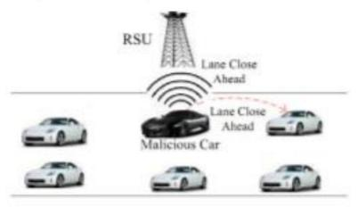
**4.2. Distributed Denial of Service (DDos):** is more severe than the DoS where a number of malicious cars attack on a legitimate car in a distributed manner from different locations and timeslots. The below figure demonstrates that three malicious black cars attack on the car A from different locations and time so that A cannot communicate with the other vehicles[4].
