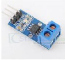
The ACS712 Current Sensors offered on the internet are designed to be easily used with micro controllers like the Arduino.
